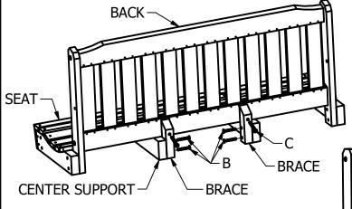
**1)** Attach Braces to Center Seat Supports using four "B" bolts.
